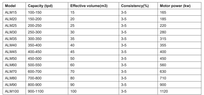
The capacity may be different according to different pulp variety and consistency. So the capacity in the above chart is only used for choosing the model.
