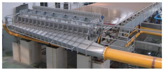
Headbox is used for sizing in fourdrinier wire section of paper making machine for producing cardboard paper, corrugated base paper, writing and printing paper, offset paper and so on.
